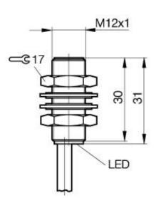
**Inductive Sensors** BES 516-329-G-E4-Y-PU-05 M12x1 x 31 normally-open Sn=4mm shielded
